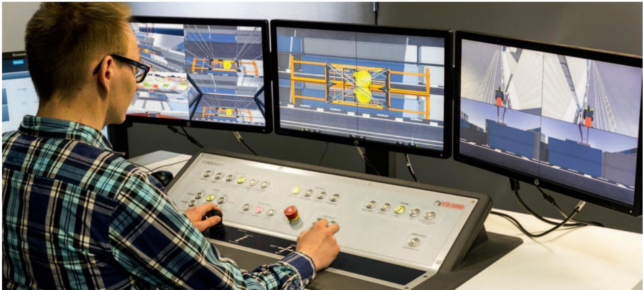
*The most significant cost savings from automation are due to the drastically smaller number of operators required. Typically, a single operator can handle two to three AutoRTGs remotely, and in quiet periods even up to six machines.*
